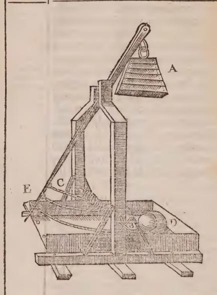
That great box or cavity at Ai, is supposed to be full of some heavy weight, and is forced up by the turning
